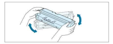
3. Reinstall the cartridge and close the cover.
